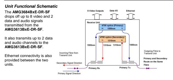
As each unit regenerates the optical signal, the optical dynamic range between each optically connected node is 17dB.
