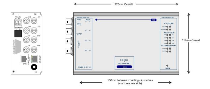
The **AMG3684BxE-DR-SF** is a standalone eight channel video receive unit designed to receive up to 8 video signals from a single fibre multimode optical fibre ring with Dual Redundant operation. It also provides 2 bi-directional data/audio channels via a low speed data interface plus full duplex 100BaseT Ethernet connectivity around the ring.
